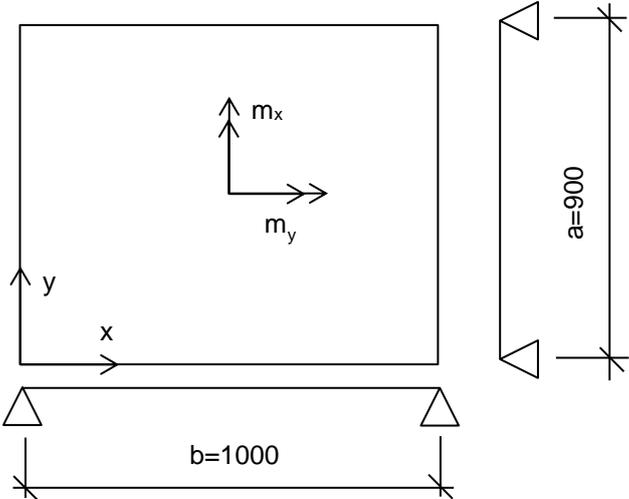
Fig. 4.1: Peripheral dimensions of the slab and its local coordinates
