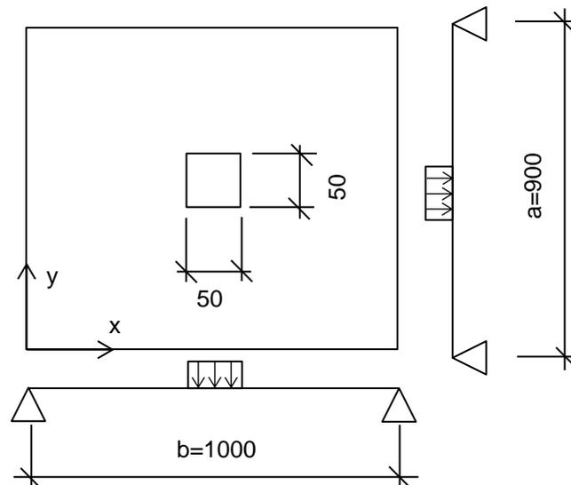
Fig. 4.4: Local load position on the slab
