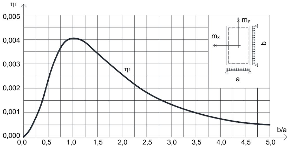
Fig. 4.8: Graph with  $\eta_f$  coefficient for vertical deflection determination caused by uniform loading, [8]
