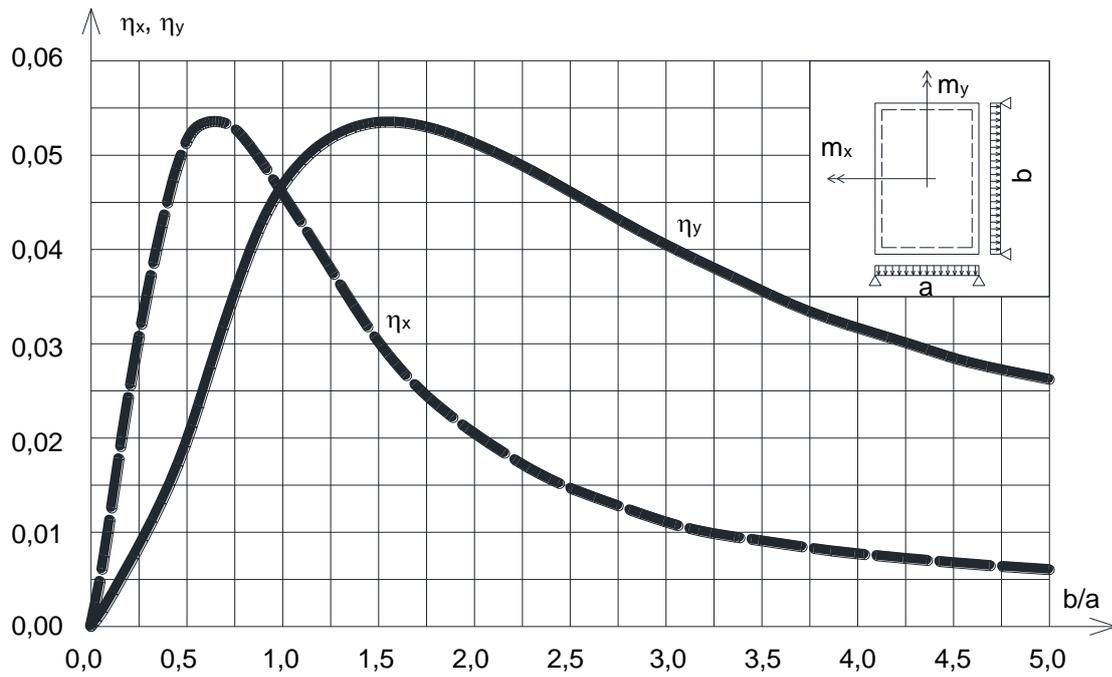
Fig. 4.6: Graph with load distribution coefficients  $\eta_x$  a  $\eta_y$  for the uniform loading, [8]
