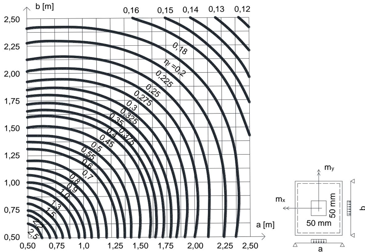
Fig. 4.9: Graph with  $\eta_{f,Q}$  coefficient for vertical deflection determination caused by local load, [8]
