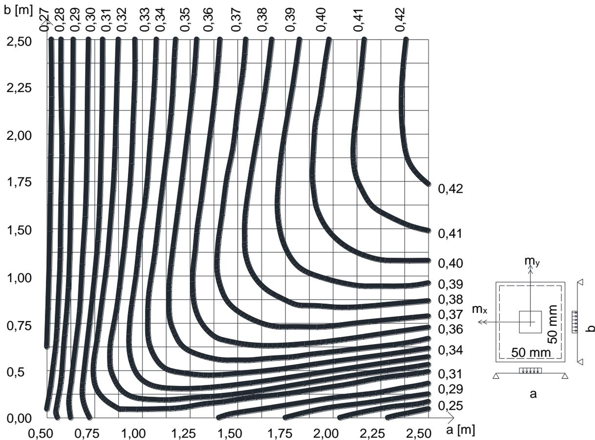
Fig. 4.5: Graph with load distribution coefficients  $\eta_{x,Q}$  for the local load, [8]
