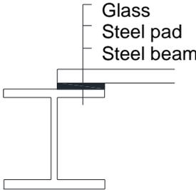
Fig. 4.2: Detail of floor slab with supporting beam's flange contact
