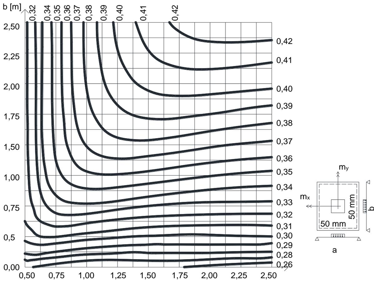
Fig. 4.7: Graph with load distribution coefficients  $\eta_{y,Q}$  for the local load, [8]
